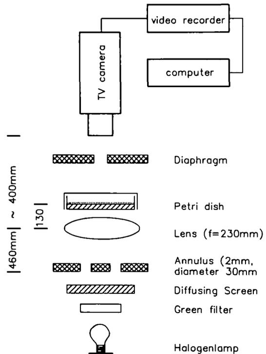
Fig. 1. Schematic diagram of the dark-field equipment.
