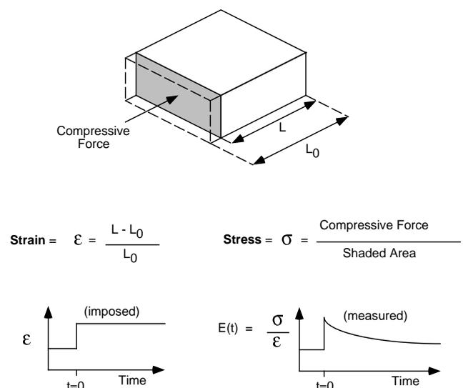
**Fig. 3.** Stress-relaxation test in uniaxial compression. A finite strain is imposed on a block of material and then held constant. The stress required to maintain the strain is recorded as a function of time and the relaxation function of the material is obtained by plotting the stress per unit strain as a function of time.
