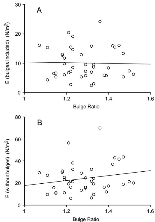
**Fig. 6.** Graphs of  $E(50)$ , calculated (A) with and (B) without including the contribution of bulges (see Fig. 5) to the explant's width and thickness when calculating stress and strain. The regression lines suggest that stiffnesses calculated by including bulges are less sensitive to the size of the bulges than stiffnesses calculated without the bulges.
