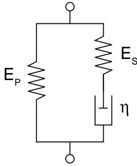
**Fig. 7.** Viscoelastic mechanical network model comprising a spring (elastic modulus= $E_p$ ) in parallel with a Maxwell element having a spring (elastic modulus= $E_s$ ) arranged in series with dashpot (viscosity= $\eta$ ).
