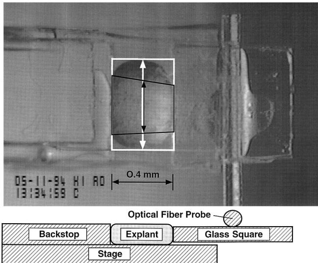
**Fig. 5.** Video image and end-view diagram of IMZ explant on Histowiggler stage showing relative positions of explant, probe with attached square of glass and stage with attached backstop. The two-headed arrows indicate the width of this explant measured when bulges on the tissue were included (white arrow) or ignored (black arrow).
